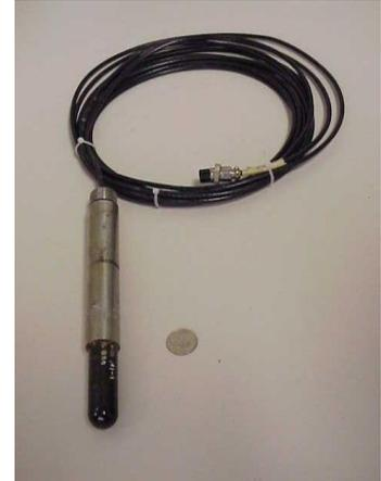
Figure 7. 1-inch diameter hydrophone
