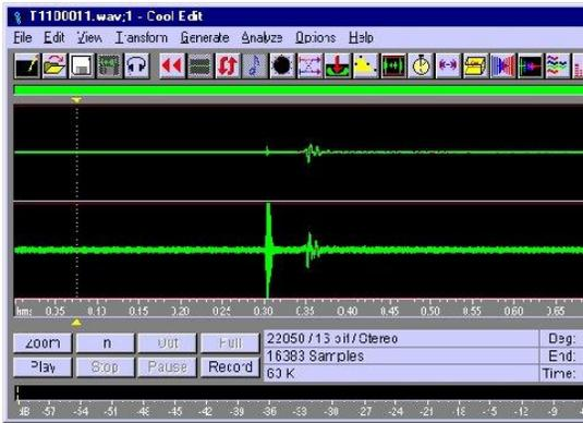
Figure 12. Time-domain graph of wire noise
