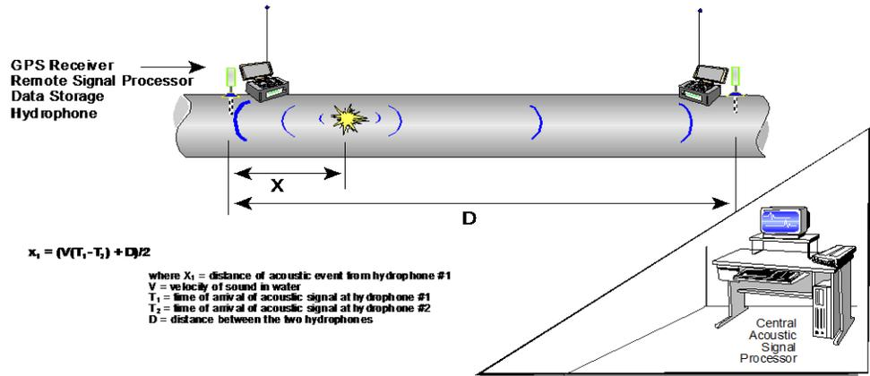
Figure 6. Schematic of autonomous test point
