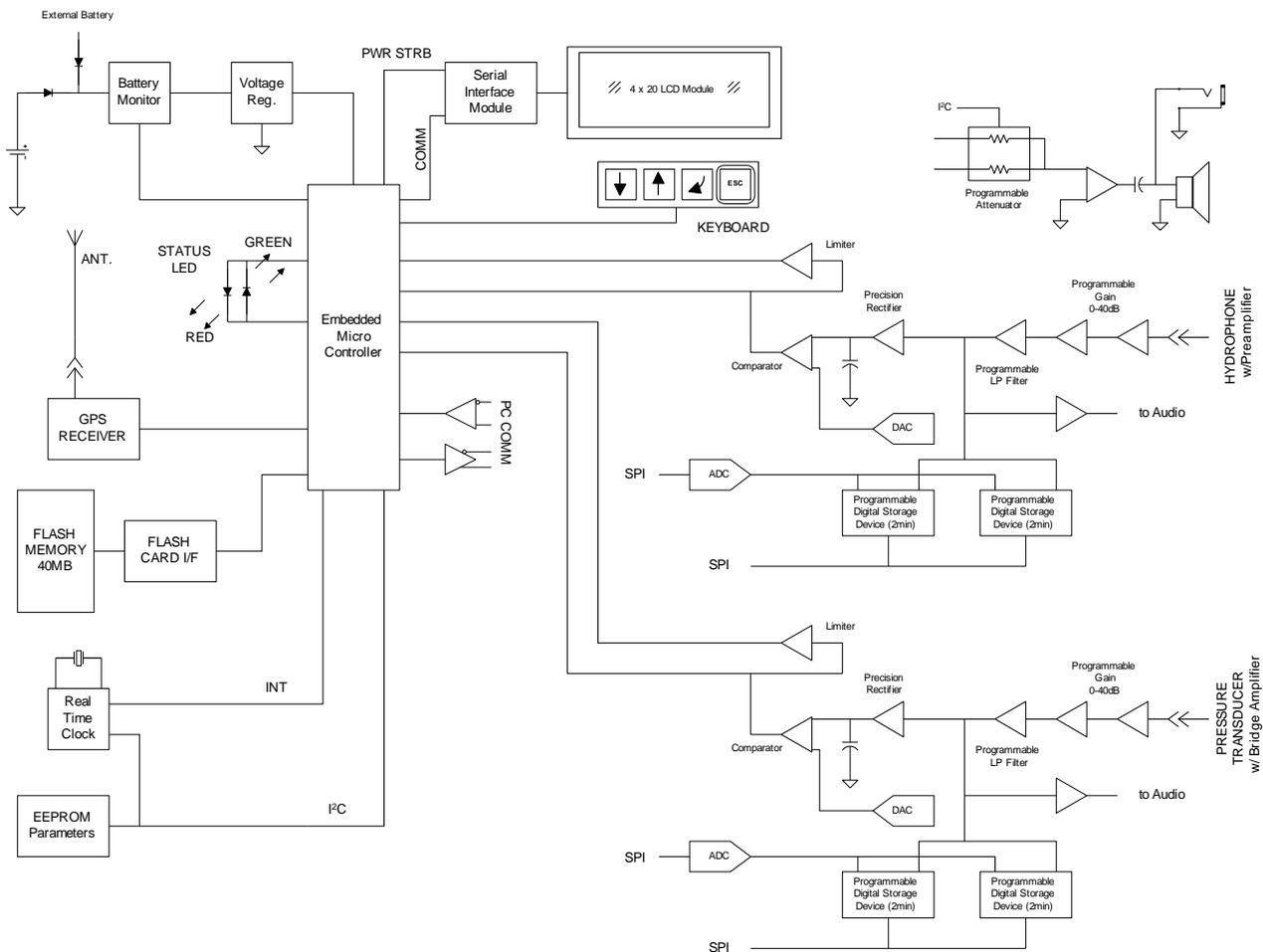
Figure 10. AH-3 Sampling system, block diagram
