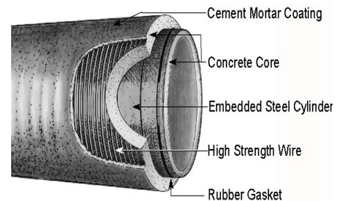
Figure 3. Cutaway view of PCCP
