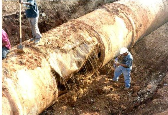
**Figure 1 – Transient-caused failure, Superaqueduct of Puerto Rico**
