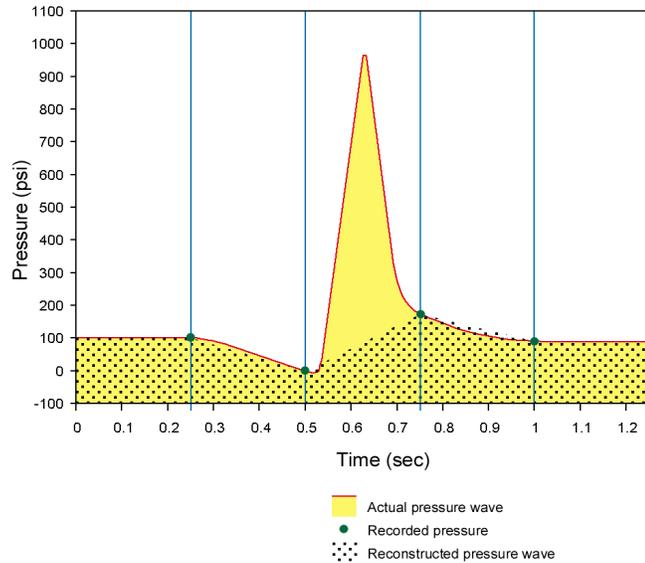
**Figure 4 – Digital data collection with insufficient sample rate**
