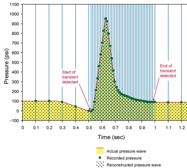
**Figure 5 – The TP1 Transient Pressure Monitoring System algorithm**
