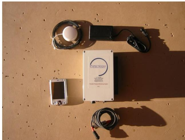
**Figure 6 – TP1 Transient Pressure Monitoring System components**
