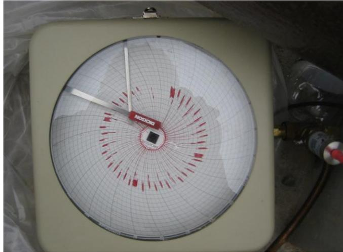
**Figure 2 – Circular graph recorder, with no negative pressure capability**
