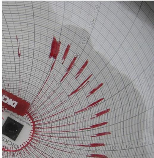
**Figure 7 – Circular graph of sewage lift station discharge pressure**
