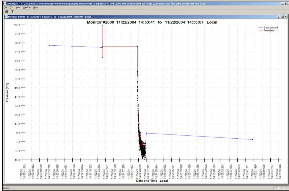
**Figure 9 – TP1 graphic depiction of the lift station pump shutdown sequence pressure (Note negative pressures to -14.5 psi)**
