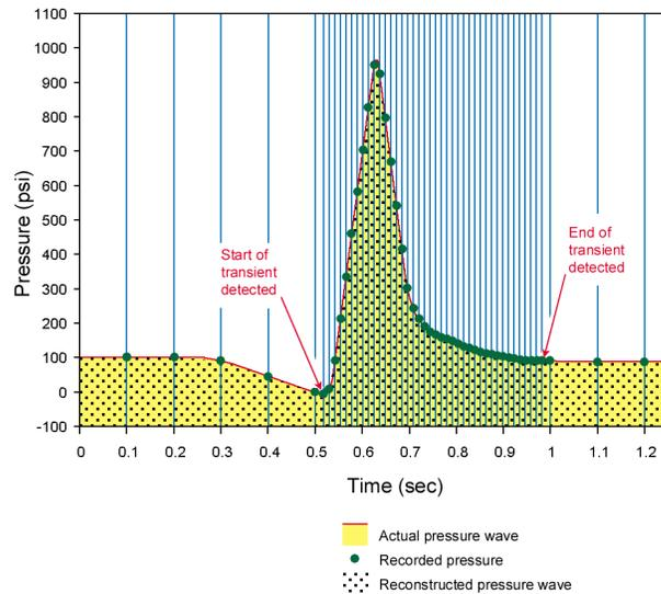
**Figure 8 – The TP1 Transient Pressure Monitoring System algorithm**
