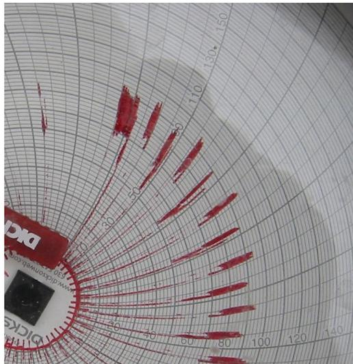
**Figure 10 – Circular graph of sewage lift station discharge pressure**
