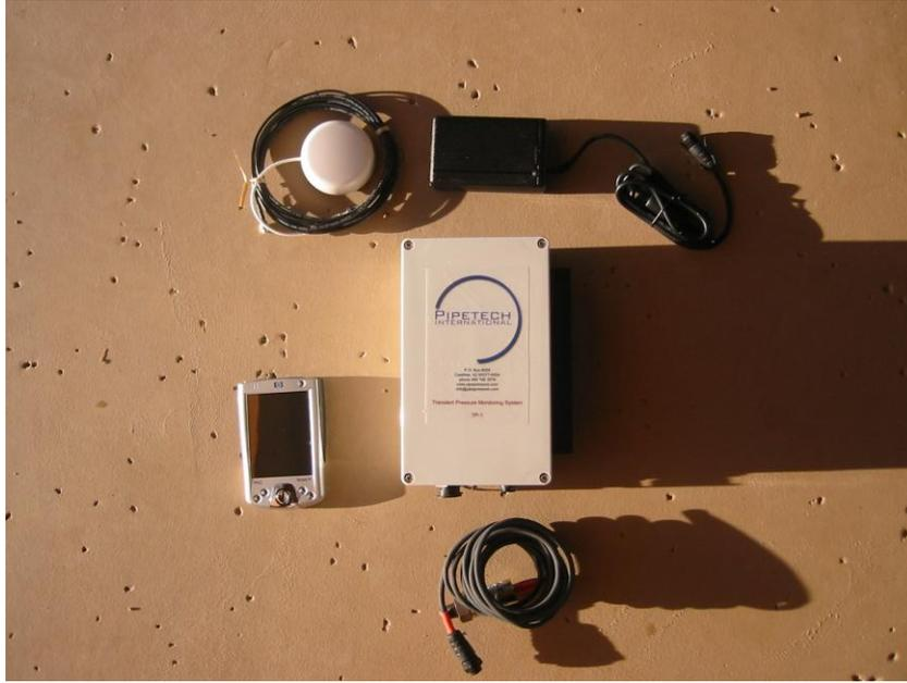
**Figure 9 – TP1 Transient Pressure Monitoring System components**
