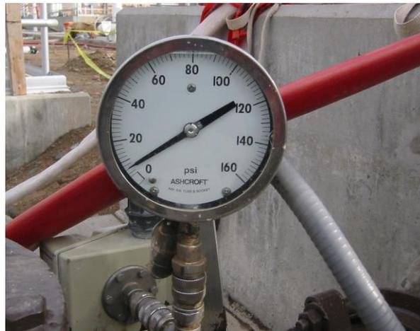
**Figure 4 – Typical pressure gauge with no negative pressure capability**
