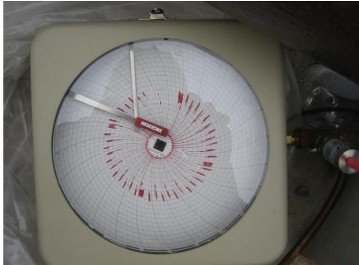
**Figure 5 – Circular graph recorder, with no negative pressure capability**
