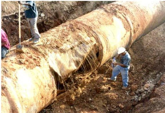
**Figure 1 – Transient-caused failure, Superaqueduct of Puerto Rico**
