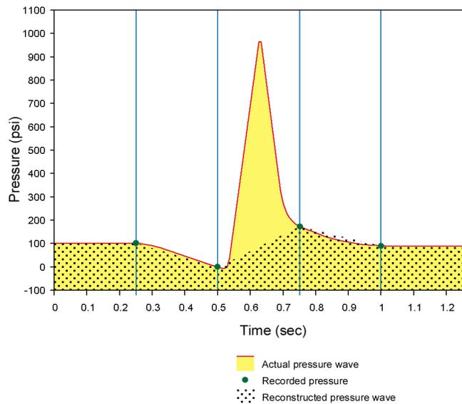
**Figure 7 – Digital data collection with insufficient sample rate**
